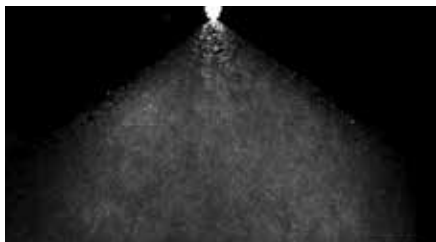
80° or 110° wide spray pattern producing a smaller droplet spectrum with a stainless steel orifice.
