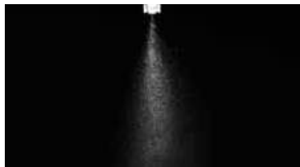
Pre-orifice design limits the formation of small droplets; reducing drift potential with a medium droplet spectrum.
