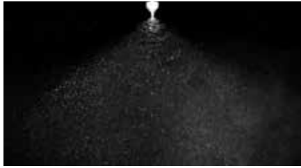
Flexible 110° air inducted spray pattern capable of meeting many spraying situations.
