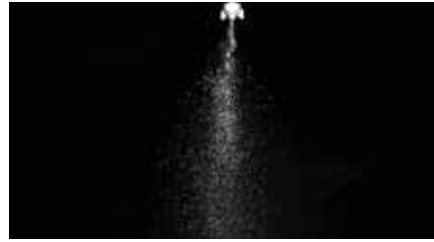
Unique 60° thick spray pattern for a wider coverage area. 120° wide by 60° thick pattern.
